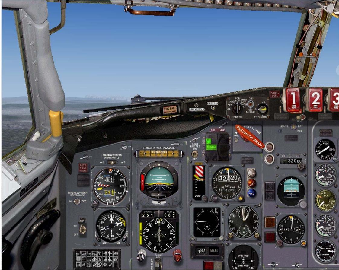
*Captain Lewis is shown here in his Boeing 727 tracking direct to the DRK VOR. VOR2 is dialed into the BCE VOR. The flight is KABQ-KSLC and is being flown by hand without the use of GPS, autopilot or FSNAV.*
