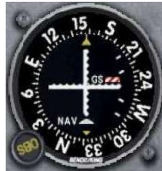
The needle is now pretty much centered – we need to turn to a heading off about 155 degrees to fly direct to this VOR. Since we are flying direct, we can even tune the VOR a degree or two to the left or the right to center it even more once we have finished the turn.
