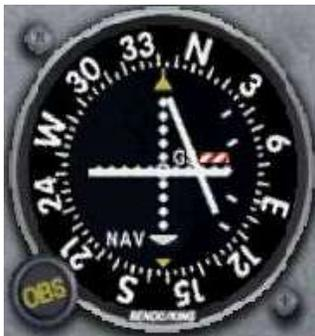
We tune in the VOR and of course the needle isn't centered, so we want to center the needle – we tune the OBS knob until the flag changes from outbound which it is showing here, to inbound
