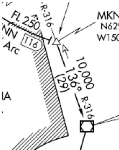
This is a Minimum Enroute Altitude. Descent below the MEA is not authorized; nor is it safe. MEAs are in place to ensure obstacle clearance, so ensure you stay above the published MEA.
