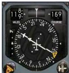
The needle finally centers on course 159; this is the direction we need to fly to go direct to the VOR.
